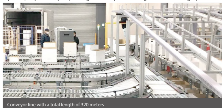
Conveyor line with a total length of 320 meters
