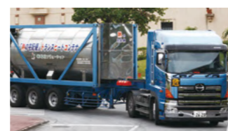
Trans-Heat Container for delivering thermal energy
