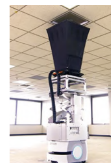
Air-flow measurement by an automated robot
