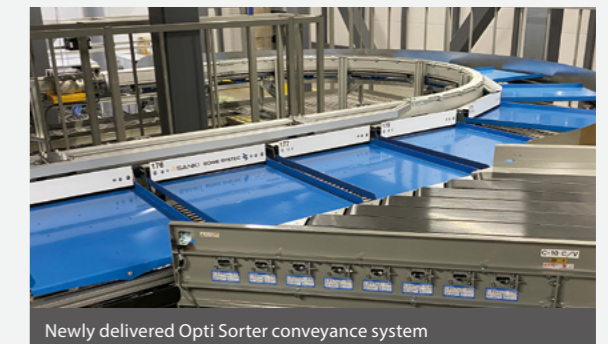
Newly delivered Opti Sorter conveyance system
