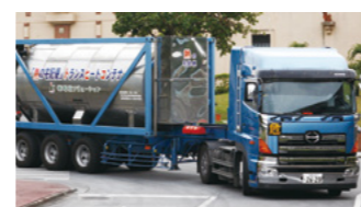
Trans-Heat Container for delivering thermal energy
