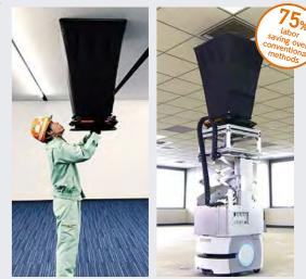
(Left) Airflow measurement by hand
