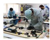
\*A new construction method whereby lightweight aluminum pipes are used instead of copper pipes, and they are connected with specialized tools to save
