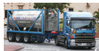
Trans-Heat Container for delivering thermal energy
