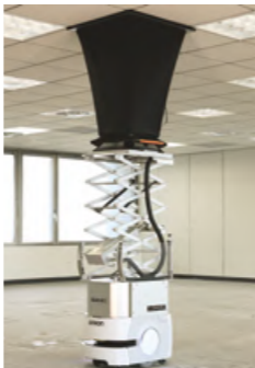
Air-flow measurement by an automated robot
