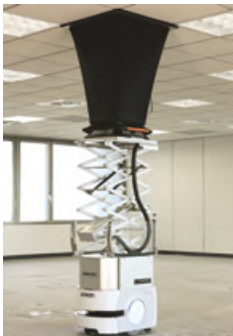
Air-flow measurement by an automated robot
