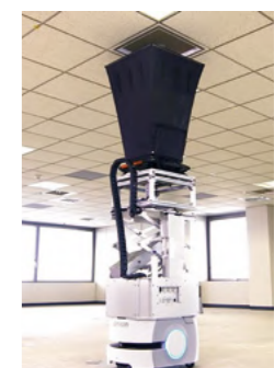
Air-flow measurement by an automated robot
