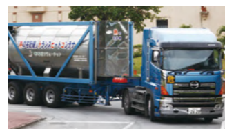
Trans-Heat Container for delivering thermal energy
