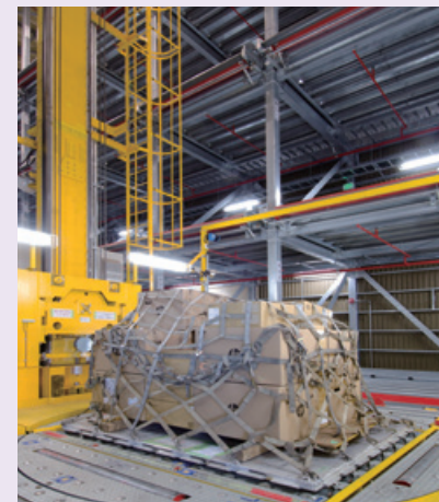
Elevating transfer vehicle (ETV) used to transport cargo
